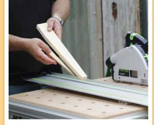
On a track saw, cut the spike according to the diagram.
