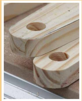
Screw the two side pieces together and then drill a 20mm hole through both using a drill and a 20mm forstner bit.
