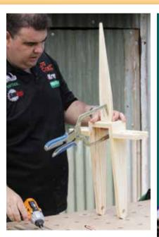
Attach all the pieces together using the Kreg pocket hole system.
