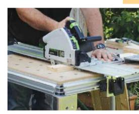
Using one of the 420mm x 90mm pieces, make a template for the uprights, as in the diagram, using the jigsaw and track saw. Rough cut the other two side pieces with a jigsaw. Once you have done this, screw the template to each of the other two 420mm pieces, one at a time, and trace out the two side pieces using the router table with a cutting bit. Keep the template for future use.
